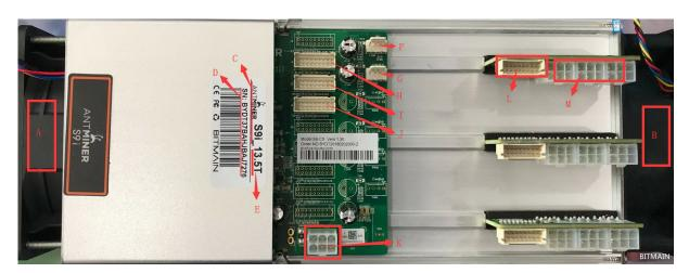
A. Front fan (intake fans); B. Rear fan (exhaust fans); C. Miner model; D. Serial number (SN) of miner, to review warranty status; E. Estimated hash rate of miner model; F. Rear fan connector; G. Front fan connector; H. Chain #8 connector; I. Chain #7 connector; J. Chain #6 connector; K. 6-pin power connector; L. Control board chain connector; M. 6-pin power connector
